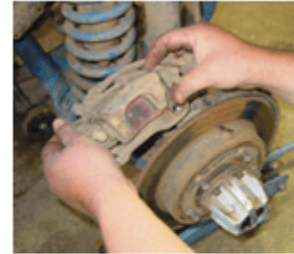
Worn brakes are usually noisy brakes. Play between the calipers and the mounts, missing or badly corroded shims, and/or missing, bent or broken anti-rattle clips and springs can all contribute to a noise problem.
