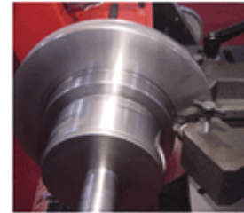
Light sanding with an abrasive disc or flexible honing brush after the rotors have been turned can improve the surface finish even more and provide an extra assurance that the rotors will remain noise-free.
